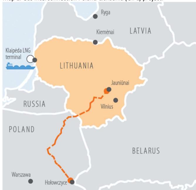
The total length of the planned gas pipeline will be 508 km, of which 165 km in the Lithuanian territory. Capacities created after construction of the gas interconnection will enable to transport annually in the direction of the Baltic States up to 27 TWh of natural gas, in the direction of Poland – up to 21 TWh annually, and the Baltic and Finnish gas markets will become a part of the single gas market of the EU.
