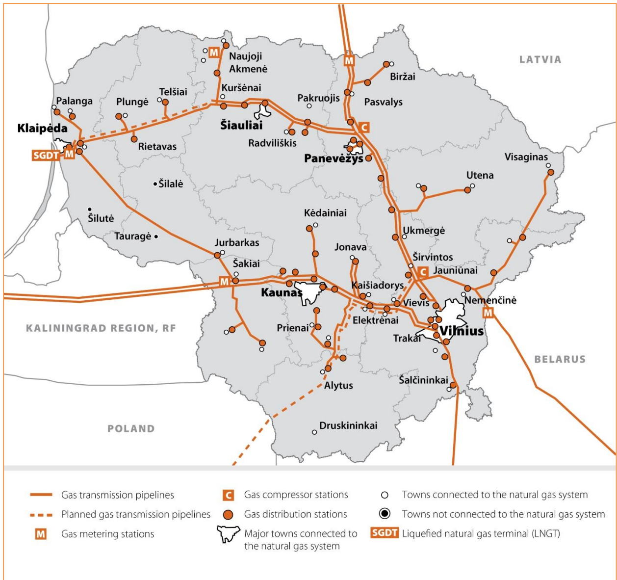
Chart No. 3. Existing Lithuania's Gas Transmission System
